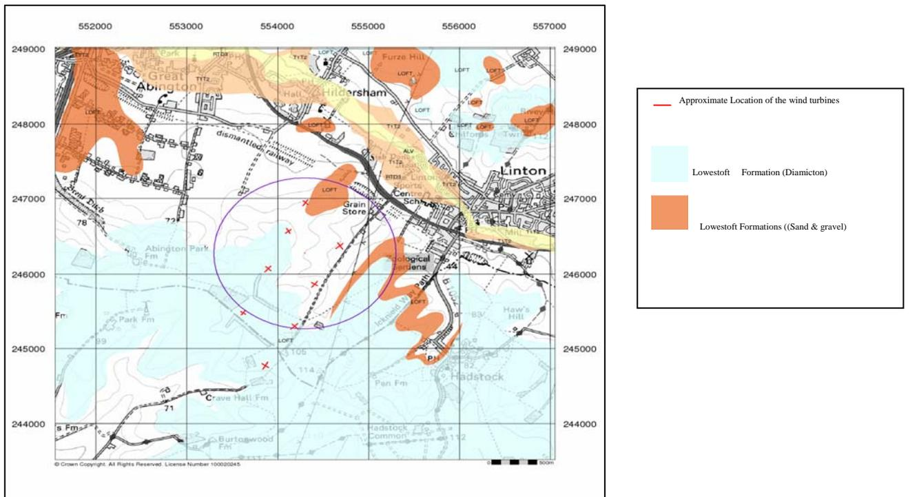
Figure 6.3 Superficial geology of the project area and approximate wind turbine locations
